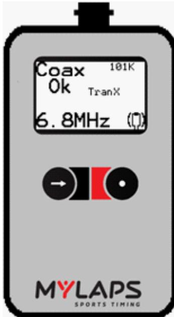
Fig. 10: LoopTester Properly connected
