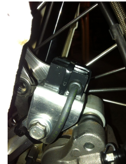
Picture 1. Radio Box on top of brake caliper.
