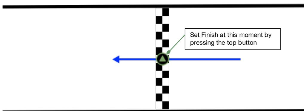
Once the finish line location is set, drive a full lap. The T DASH XL will 'draw' the track live including the finish line position. After 1 full lap the current track position will be shown by a red dot.
